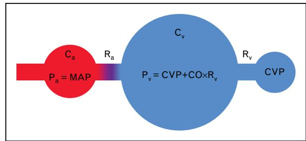
**FIGURE 1.** Lumped circulatory model consisting of an arterial ( $C_a$ ) and a venous ( $C_v$ ) capacitance connected by arterial ( $R_a$ ) and venous ( $R_v$ ) resistances.  $C_v/C_a=24$  and  $R_a/R_v=25$  [30].
